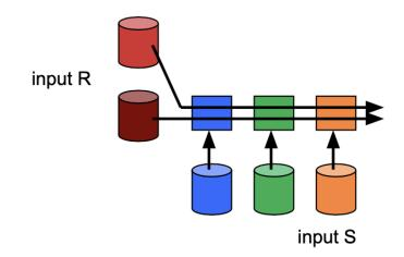
For instance, if relation R is small, we could do a broadcast join by sending R to all machines that have a partition of S. We perform a local join at each machine and union the results.
