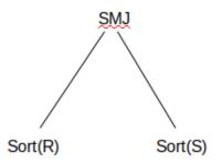
One machine can work on sorting R and another machine can sort S at the same time. In interoperator parallelism, we parallelize the entire query, not individual operators.
