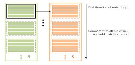
The I/O cost of this is somewhat better. It's [R] + [R][S] – this can be optimized by keeping the smaller relation between R and S as the outer one.
