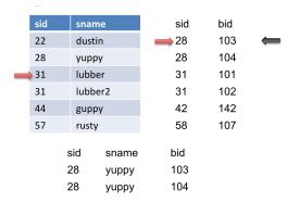
We will advance the pointer (the red arrow) on S because 28 < 31 until S gets to sid of 31. Then we will mark this record (the black arrow). In addition, we will output this match.
