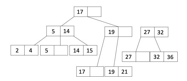
Since it was an inner node that overflowed, we will **MOVE**  $L_2$ 's first entry up to the parent and adjust pointers to get:
