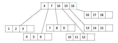
In the figure above, we see that the parent node has overflowed. We will split the parent node into two nodes and create a new parent:
