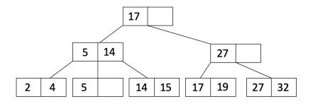
Now let's insert 21 into our tree. When we insert 21, it causes one of the leaf nodes to overflow. Therefore, we split this leaf node into two leaf nodes as shown below:
