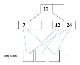
In the figure above, if we want to read records with 12 and 24, then we would have to read in each of the data pages they point to in order to retrieve all the records associated with these keys.
