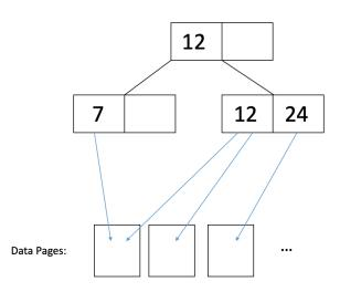
In the figure above, we can read records with 7 and 12 by reading 2 pages. If we do sequential reads of the leaf node values, the data page is largely the same. In conclusion,
