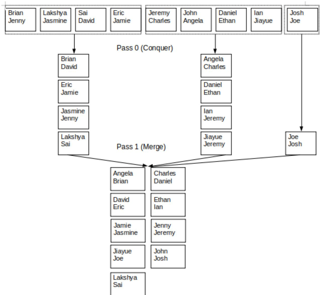
Now we take in 4 pages at a time during the conquering phase and output a sorted run of length 4. In the merging pass, we can merge all three sorted runs produced during the conquering pass at once. This cut the number of passes (and thus our I/Os) in half!
